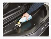
Once the mixture has been prepared, it is necessary to open the front cargo area and unscrew the cap on the right side of the vehicle. Pour the detergent water mixture until it fills to level. Be sure to close the cap once filling is complete.
