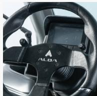
**Drive command ("D").** When the button identified with the letter "D" is activated, the vehicle moves forward, using the accelerator pedal.
