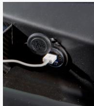
**USB charger socket.** The USB charger socket on the passenger side is activated using the built-in button. You can charge, for example, two devices simultaneously. The charging capacity is 2.1 amperes per duct. The socket also works if the vehicle is "OFF".
