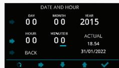
**Date and Hour:** selecting this item, you can adjust the date and time on the display. Move on the data to edit using the keys under the arrows. The circular arrow allows you to go from one line to the next. To return to the main menu, the BACK item must be pressed.
