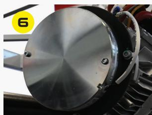
4. tight the supplied M5x30 screws in each hole to compress the internal springs and allow the clutch disc to rotate freely (photo 5 - 6).
