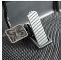
**Brake pedal.** There is redundancy on the brake pedal. In case of an emergency, by pressing the brake pedal traction is disabled.
