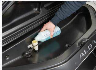
Once the mixture has been prepared, it is necessary to open the front cargo area and unscrew the cap on the right side of the vehicle. Pour the detergent water mixture until it fills to level. Be sure to close the cap once filling is complete.
