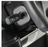
**Steering wheel height adjustment lever.** Placed under the steering column, when activated, it allows you to adjust the height and length of the steering wheel according to the driver preferences. At the end of adjustment, return the lever to the locking position of the column.
